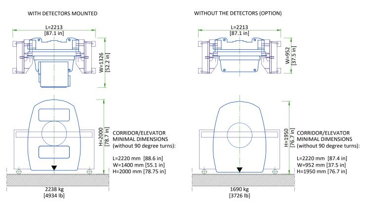
THE GANTRY IS SHIPPED ON A DOLLY EQUIPPED WITH ELEVATING CASTERS (NORMAL SHIPPING CONFIGURATION).
