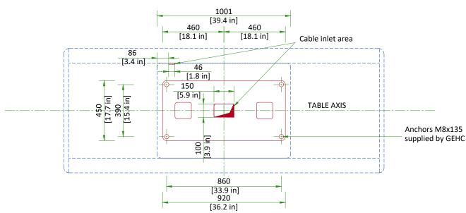
The floor bearing the system is recommended to be concrete and the thickness to be determined by a Structural Engineer to properly support the equipment loads. The supplied anchors require a minimum embedment of 90 mm [3.5 in] into the concrete. If the floor thickness is less than 95 mm [3.7 in], it is recommended that the unit be secured using a through-bolt method with a reinforcement plate on the back side.
