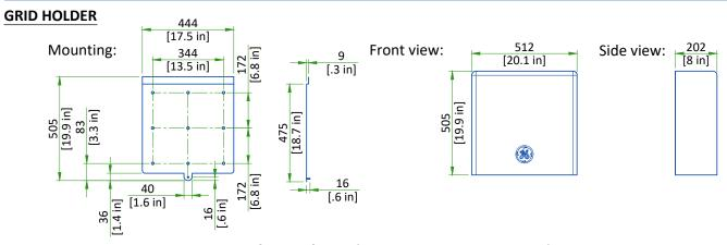
Grid Holder should be installed 10cm to 20cm [4in to 8in] height from the Grid Holder bottom to the floor.
