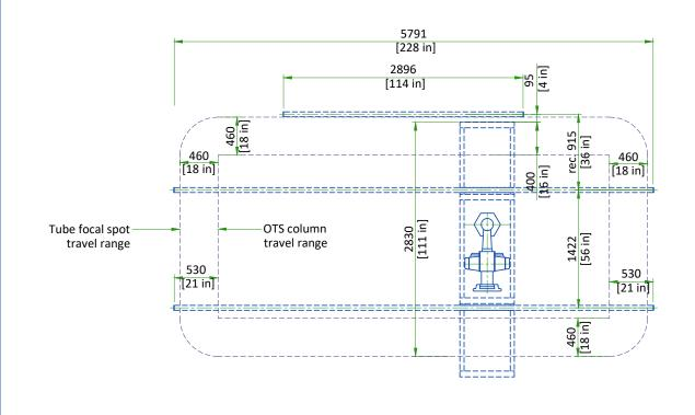
NOT TO SCALE Note: Focal Spot Travel depends on the length of the bridge, rails and position of bridge.
