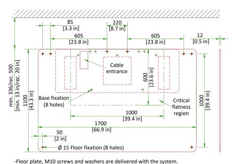
• shims may be used along perimeter of baseplate to improve surface contact
