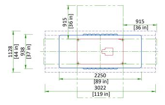
Recommended required service access clearance is 915 mm [36 in]. Minimum required service access clearance is 610 mm [24 in].
