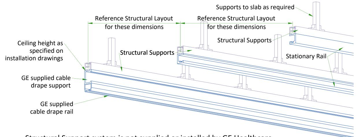
Structural Support system is not supplied or installed by GE Healthcare
