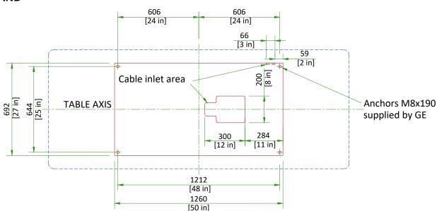
The floor bearing the system is recommended to be concrete and the thickness to be determined by a Structural Engineer to properly support the equipment loads. The supplied anchors require a minimum embedment of 90 mm [3.5 in] into the concrete. If the floor thickness is less than 95 mm [3.7 in], it is recommended that the unit be secured using a through-bolt method with a reinforcement plate on the back side.
