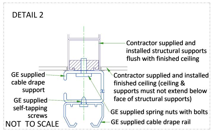
Typical | DISCOVERY XR 656 | EN-RAD-TYP-XR\_656\_(G1)-NF.DWG | Rev A|Date 07/Mar/2024 | S4 - Structural Details (2) | 10/16
